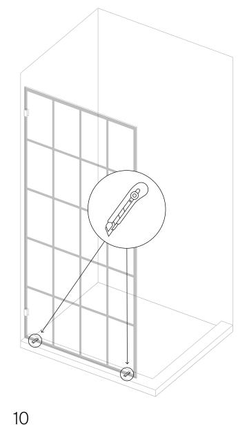
Install and level Fixed Panel into Wall Clips and onto Rubber Blocks.
